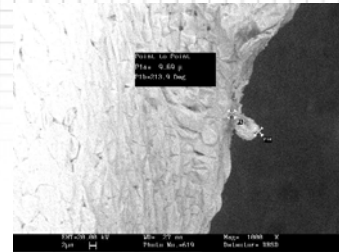
MQFP (PB-free reflow) MAX Whisker : 9.69um
